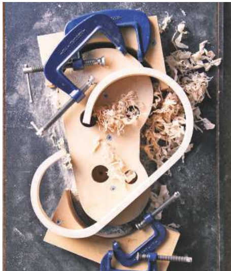
Strength in numbers: uncramped and cleaned up, the laminations created a strong and beautiful set of curves
